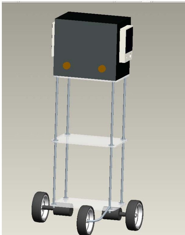
Figure A4 – Rear View of Robot with Third Wheel
