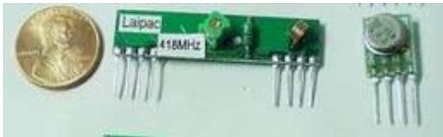
Figure 12 - Laipac Technologies™ RF Transmitter (left) and Receiver (right)
