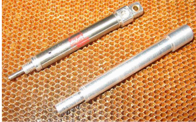
Fig. 26. A photograph of a Bimba pneumatic piston, and a corresponding machined cylinder for carbon fiber layup tests. The background is the honeycomb core used in the carbon fiber composites structures that comprise the Good Samaritan chassis.
