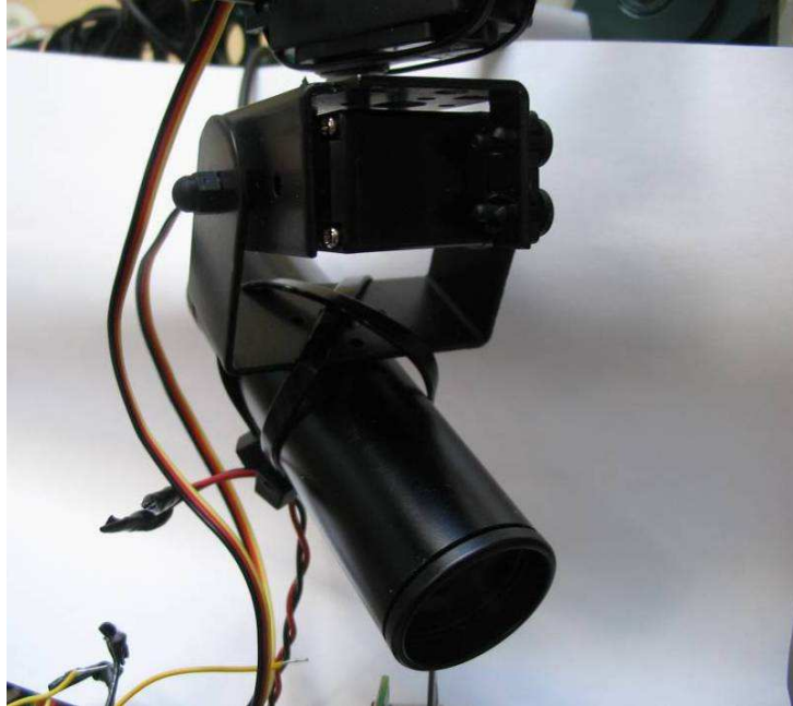
Fig 3. The Zerolux camera is mounted on two servos for multidimensional orientation control.
