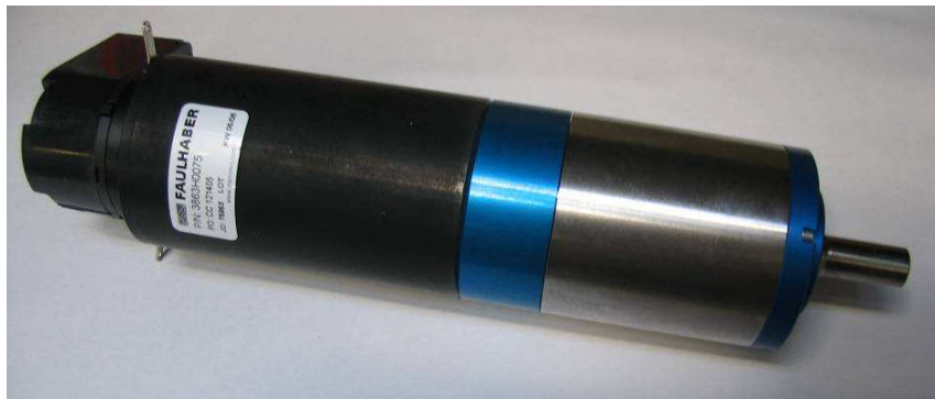
Fig. 25. Faulhaber brushed DC articulation motor with gearhead and optical shaft encoder.
