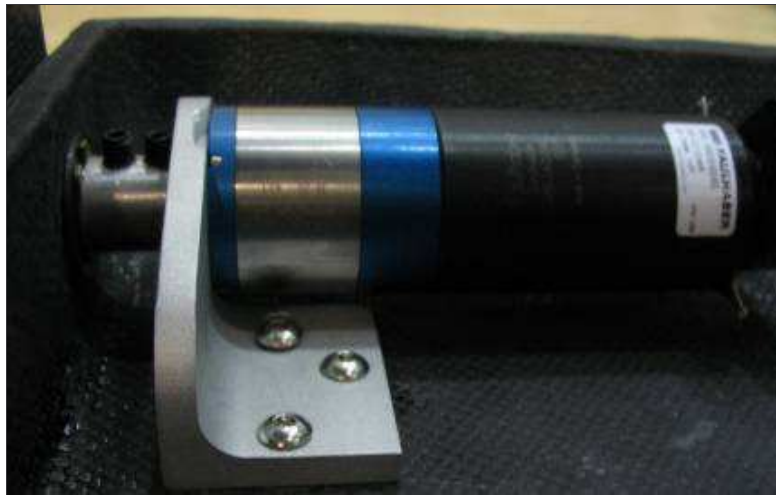
Fig. 22. Good Samaritan Chassis #1: A Faulhaber drive motor is mounted in the chassis of robot. Wiring and circuitry have been removed.
